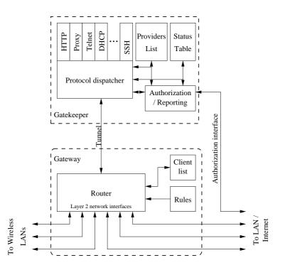
Figure 2: Block diagram of the Uni-Fy system
